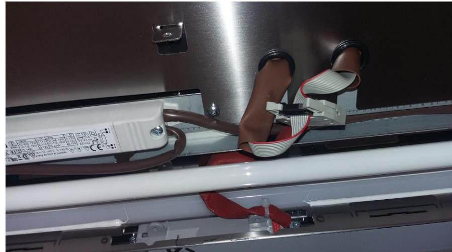
Remove the lamp support panel to get access to the lamps and to the user interface /
