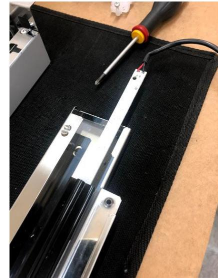
Remove 1 screw and pull out the led module lamp / Rimuovere la vite ed estrarre la lampada led
