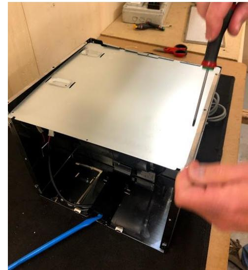
Remove 7 screws from cover panel (upon the box) and 7 screws from the back of the motor box /
