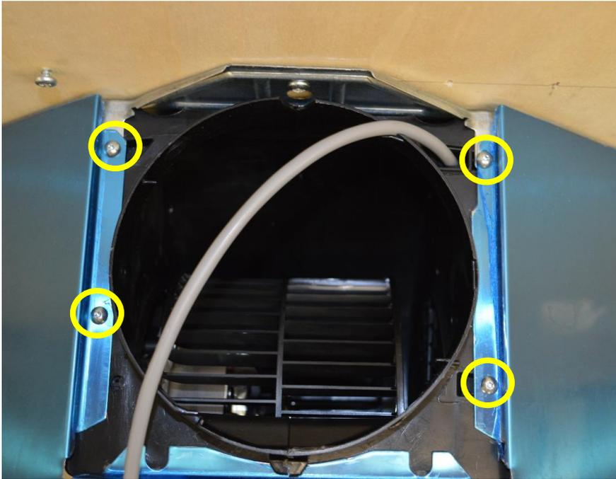
Unscrew 4 screws at the top of the product and remove the motor from the below. Be careful not to drop it, keep it from below! /
