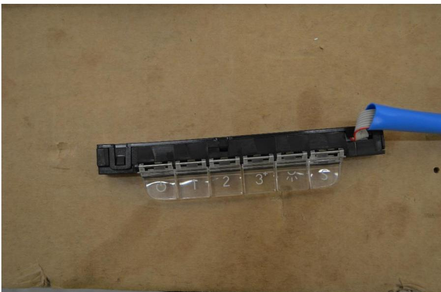
**NB: replacing the UI pay attention to the correct connection /**
