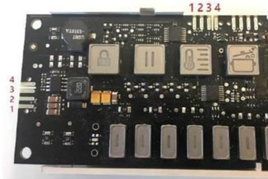
PIN EDGE CONNECTOR RAST 2.5mm
