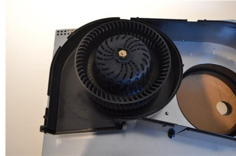
Hold the fan wheel in order to not deform it during the unscrewing. / Tenere la girante per non
